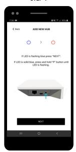
Refer to hub. If LED on top is flashing blue, select NEXT in the app. If it is solid blue, press & hold the hub's P button until it flashes, then select NEXT.
