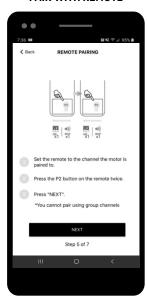
To pair with remote, select device's channel (not channel 0 and shades cannot be grouped). Remove remote battery cover. Press upper left P2 button twice until motor responds. Select NEXT.
