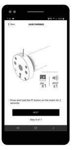
To pair with hub, press and hold the programming button on the motor head until the motor responds, then select NEXT.
